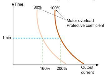
Fig 5-28 Motor overload protection curve
