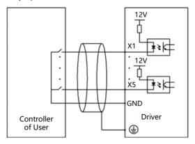
Fig.3-11 NE200 control circuit wiring diagram
