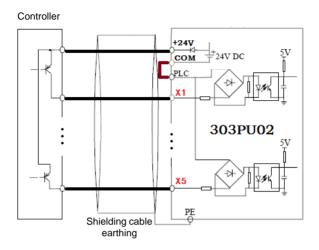
Fig. 9-3 PNP wiring diagram (Using internal power)
