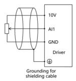
Fig.3-14 NE200 wiring diagram for analog input
