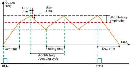
Fig.5-27 Wobble frequency running diagram
