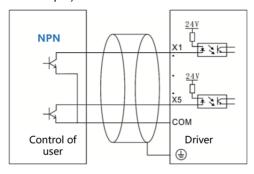
Fig.3-18 NE300 NPN common emitter wiring diagram
