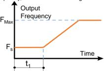
Fig.5-3 Start frequency and Start frequency holding time
