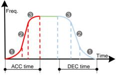
Fig.5-4 S-curve acceleration/deceleration
