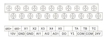
Fig.3-16 Control circuit terminals diagram
