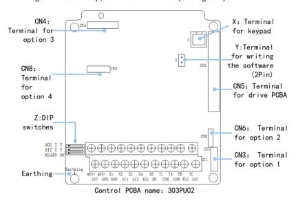
Fig. 9-1 NE300 close-loop control PCBA diagram
