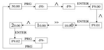
Fig.4-2 Example of 3 levels menu operating
