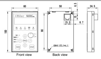
Fig.8-7 LED Operating Panel Outline and Mounting Dimension
