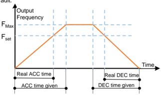
Fig.5-2 Schematic diagram for acceleration/deceleration time
