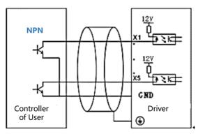
Fig.3-12 NE200 NPN common emitter wiring mode
