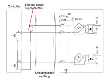
Fig. 9-5 NPN wiring diagram (Using external power)
