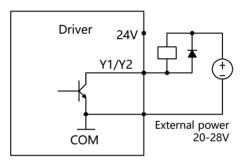
Fig.3-20 External power supply wiring mode
