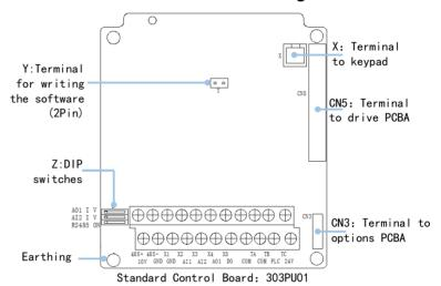
Fig.3-25 Control board schematic drawing
