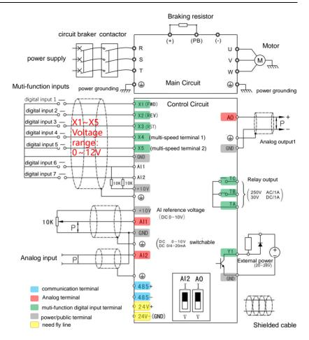
Fig.3-8 Control Terminal Wiring of NE200(Example: 0022GB~0040GB)
