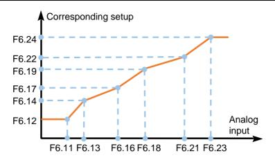
Fig.5-18 Analog input non-linear curve
