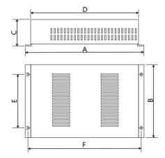
Table for dimension and weight of braking resistor
