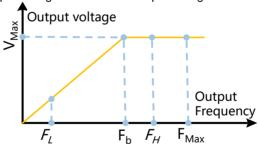
Fig.5-1 V/F characteristic diagram
