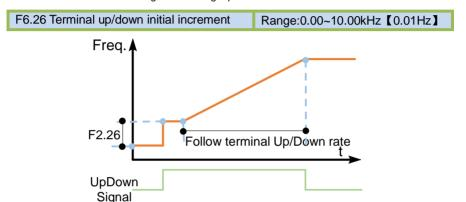
Fig.5-20 Terminal up/down initial increment
