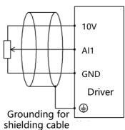
Fig.3-21 Wiring mode of analog input terminal
