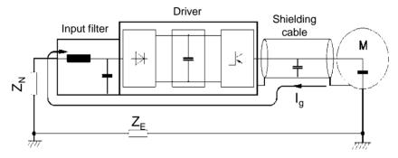
Fig.2-2 Countermeasures for Conduction and Radiation Interference
