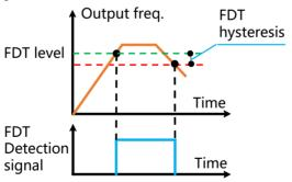
Fig.5-22 FDT level and lag diagram
