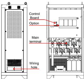
Fig.3-7 NE300 3P 400V 560~800kW(G)/630~900kW(P)
