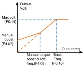
Fig.5-11 Schematic Diagram for torque boost
