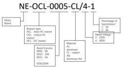
Fig. 9-6 Reactor model description
