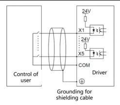
Fig.3-17 NE300 dry contacts wiring diagram for external controller
