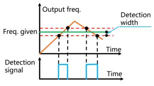
Fig.5-21 FAR detection diagram
