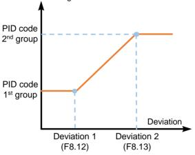
Figure 5-24 PID parameters switching
