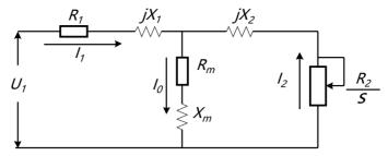
Fig. 5-13 Asynchronous motor equivalent circuit
