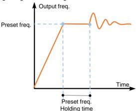
Fig. 5-25 PID preset frequency and holding time
