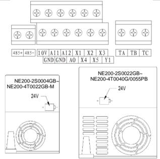
Fig.3-10 Arrangement of Control Circuit Terminals
