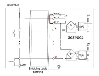
Fig. 9-4 NPN wiring diagram (Using internal power)
