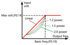
Fig.5-9 Torque-reducing curve
