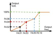
Fig.5-10Multi-points V/F curve
