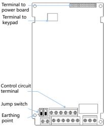
Fig.3-23 NE200 Control board schematic drawing
