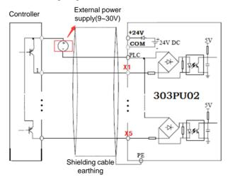
Fig. 9-2 PNP wiring diagram
